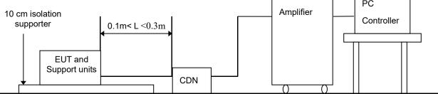
For the actual test configuration, please refer to the related item – Photographs of the Test Configuration Note: 1) The EUT is setup 0.1 m above Ground Reference Plane
